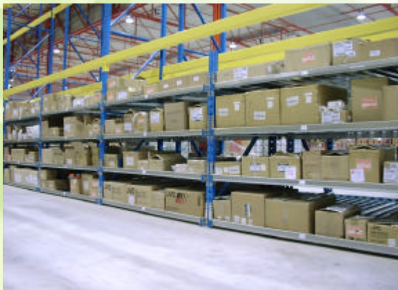
Flow rack for small item
